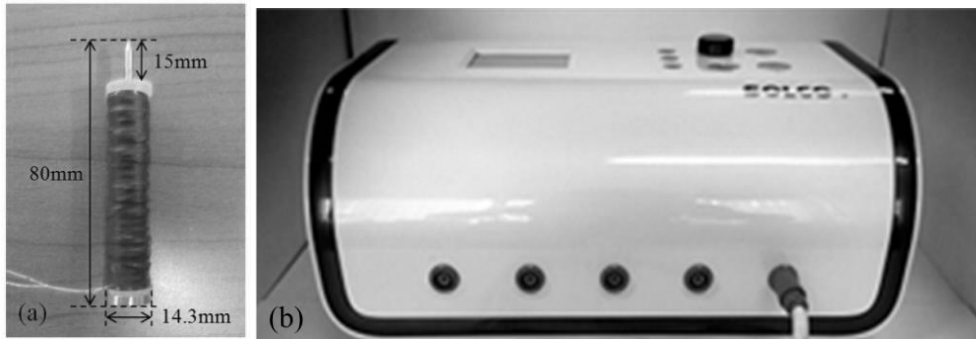
Fig. 2: (a) Electrode for generating magnetic flux. (b) Designed system.
