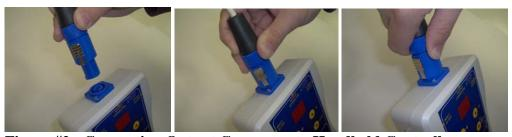
Figure #2: Connecting Output Connector to Handheld Controller
