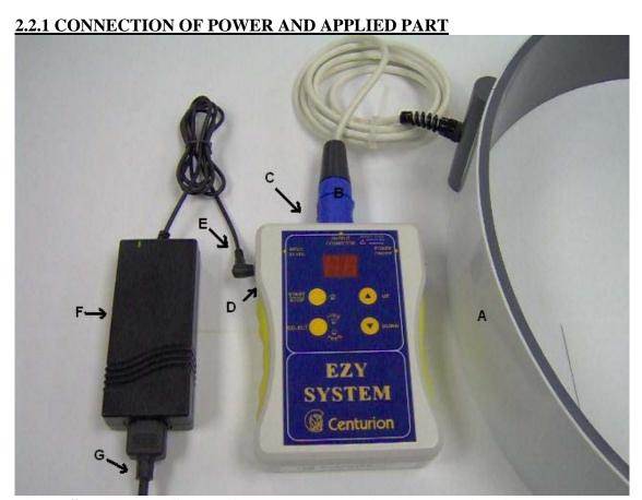
Figure #1: The EZY System Controller, Power Adapter and Applied Part
